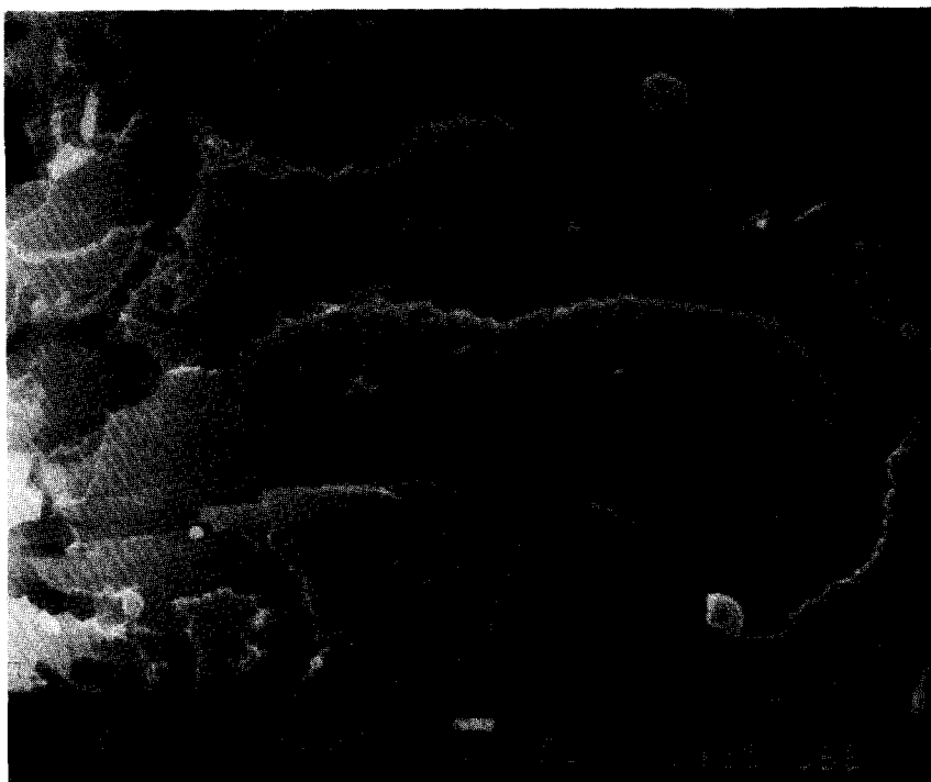
FIG. 1. SEM picture of a deep-channeling platinum particle on the basal plane of graphite after reaction with 1 atm H_2 at 1050^\circ C for 7 h and 17 min.
